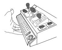
To apply legends for the function keys, pry up carefully, but with force, on the panel cover, place the legend strips above the keys. Insert the top of the panel cover first, and snap the bottom back into place.
