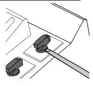
To remove wiper and light switch caps for labeling, insert a thin bladed screwdriver into the slot on either side of the switch and carefully pry up until the switch cap pops off.
